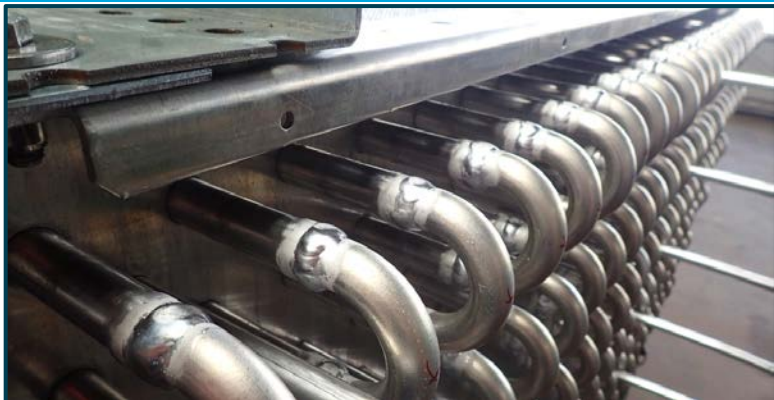
Smaller tubes for reduced \text{NH}_3 inventories
