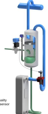
Thermosiphon system with both a Vapor Quality Sensor in the evaporator outlet and a level sensor in the separator.
