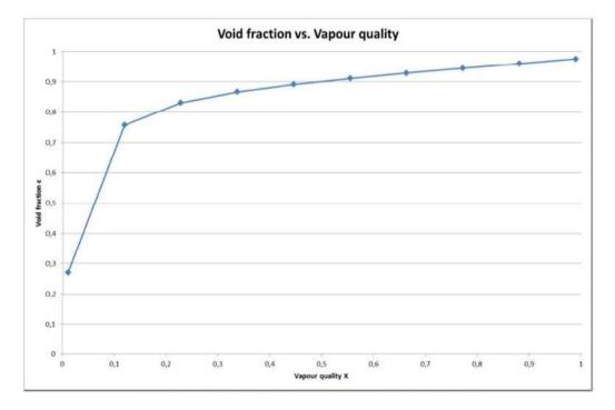
Figure 2: Void Fraction compared to vapor quality
