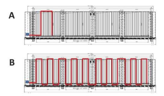
Figure 26: Shows the defrost sensor mounted on an air cooler.
