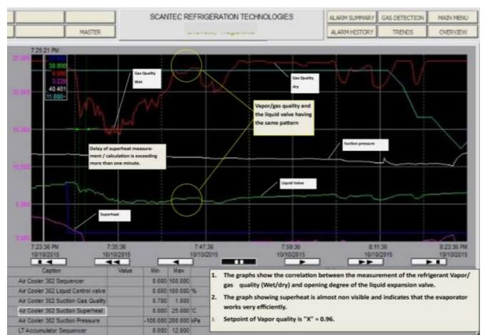
Figure 16: Graph of a DX controlled air-cooler/evaporator.
