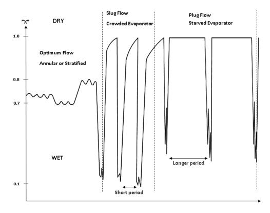
Figure 3: Shoving sensor response to a changing flow pattern and phase shift
