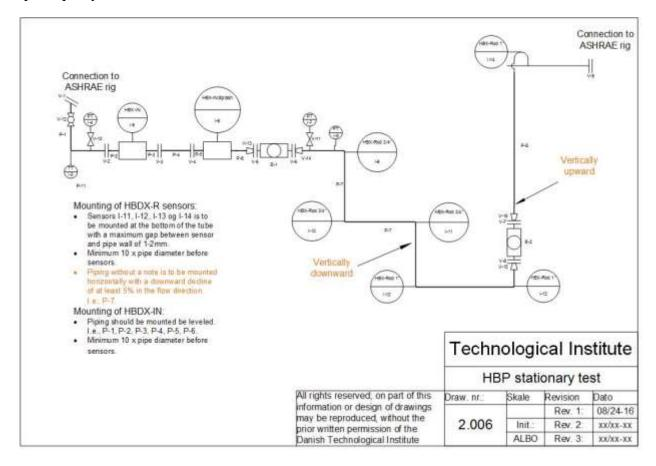
Figure 12: PI diagram for the Laboratory testing.
