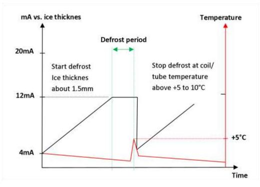
Figure 25: Operating principle of the defrost sensor.
