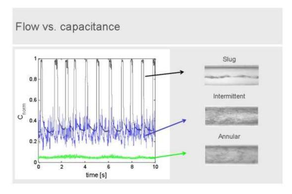
Figure 4: Flow vs. Capacitance (C nom is capacitance value in pF)
