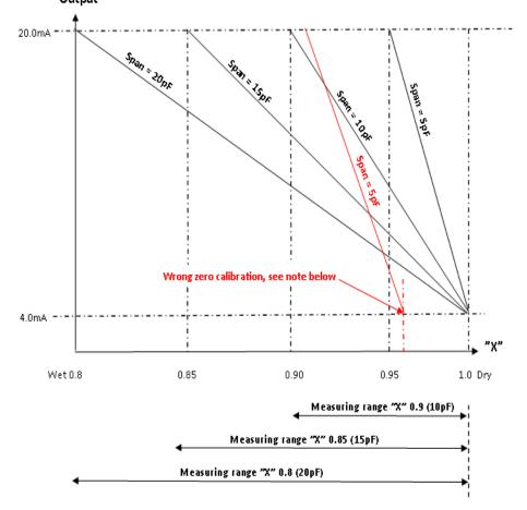
Figure 11: Graphical view of the relationship between X and span settings in pF for a HBX-DX <sup>3</sup>/<sub>4</sub> L192mm sensor.
