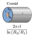
The measured value is dependent upon the total sensing area and the internal distance between the conductors/electrodes. The ratio of the capacitance measured in pF is then dependent upon the material between the electrodes. Relative permittivity is the factor by which the electric field/charges on the electrodes is changed and named as dielectric constant  $\epsilon$ , Refrigerant have  $\epsilon > 1$ , some common values are given in the table " $\epsilon$ " DC below.
