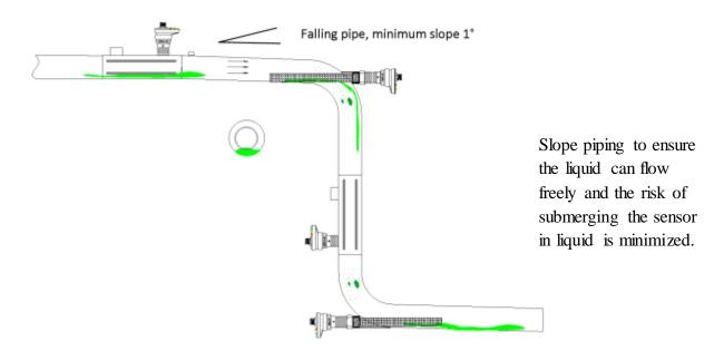
Figure 10: Recommended installation methods for rod and in-line sensor. Output
